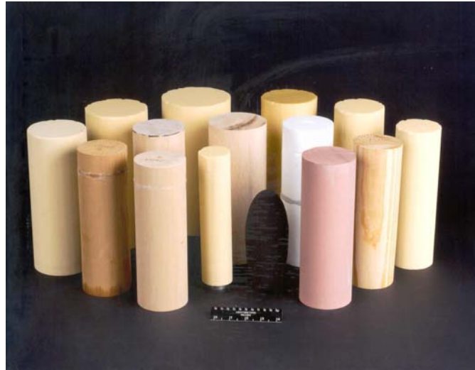
FIG. 1. The family of tested windscreens.
