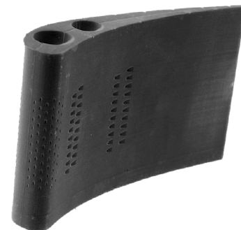
Figure 3.—Film cooled vane.
