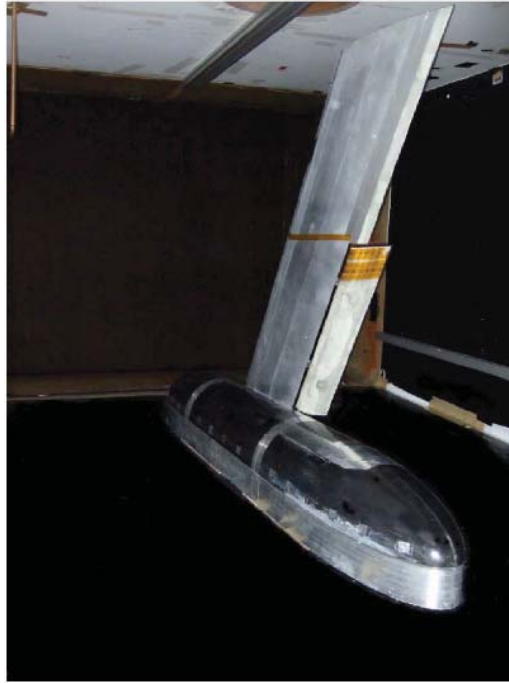
Fig. 8. Photograph of the SCCH-model used in the experimental study at the Berlin University of Technology, installed in the ISTA 2m×1.41m closed loop return wind tunnel. Inboard flap deflected to 32° (landing configuration).
