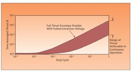
**Time-Averaged Thrust** was calculated theoretically for a representative ion thruster operating in continuous and pulse modes. A minimum average thrust much lower than that attainable in continuous operation (about 1  $\mu$ N, below which the thrust due to ion flux is comparable to the flow of the propellant gas without ionization) would be achieved by pulsing at a low duty cycle.
