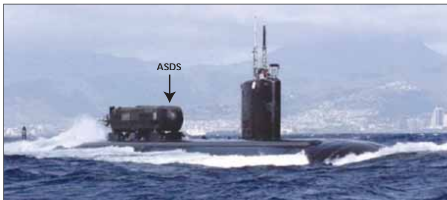
Figure 1. A Miniature Submarine, denoted an ASDS as explained in the text, rides piggyback on a submarine of the Los Angeles class.
