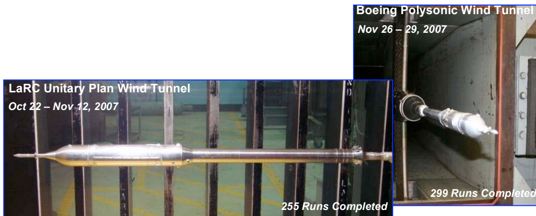
Fig. 11. Sample Ares I wind tunnel testing configurations.
