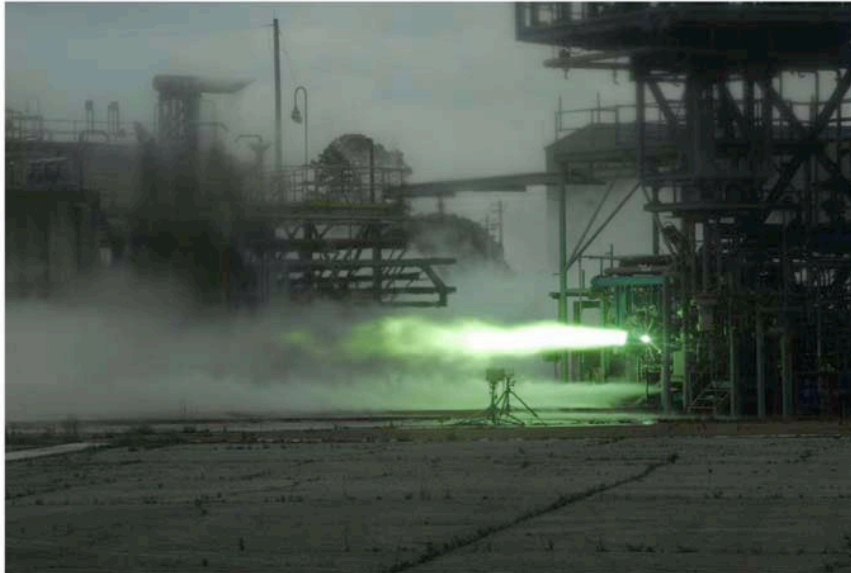
Fig 12. J-2X subscale main injector hot-fire testing at Marshall.
