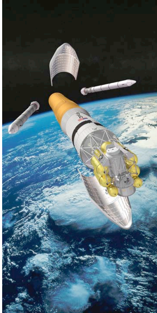
Fig. 3. NASA concept of the Ares V and Altair in Earth orbit.
