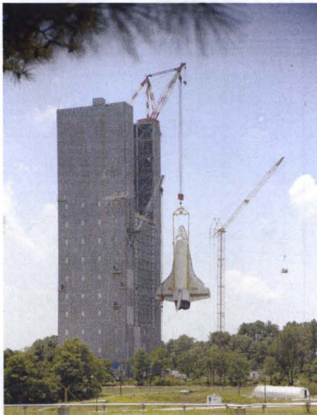
Fig. 3. The Space Shuttle was structurally tested in the Marshall Center's Dynamic Test Stand, which will be used for the Ares I integrated stack testing.
