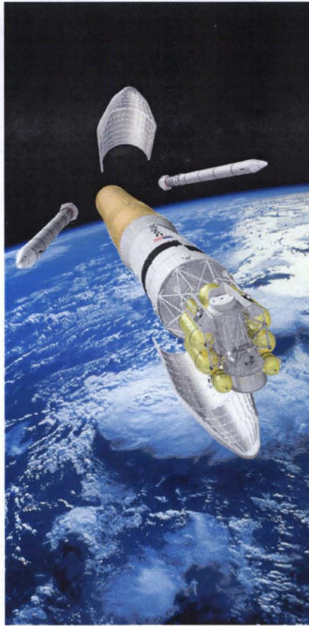
Fig. 2. The heavy-lift Ares V will transport the Altair to low-Earth orbit; its Earth departure stage will place payloads and the mated Orion crew capsule into lunar orbit in the 2020 timeframe (NASA concept).
