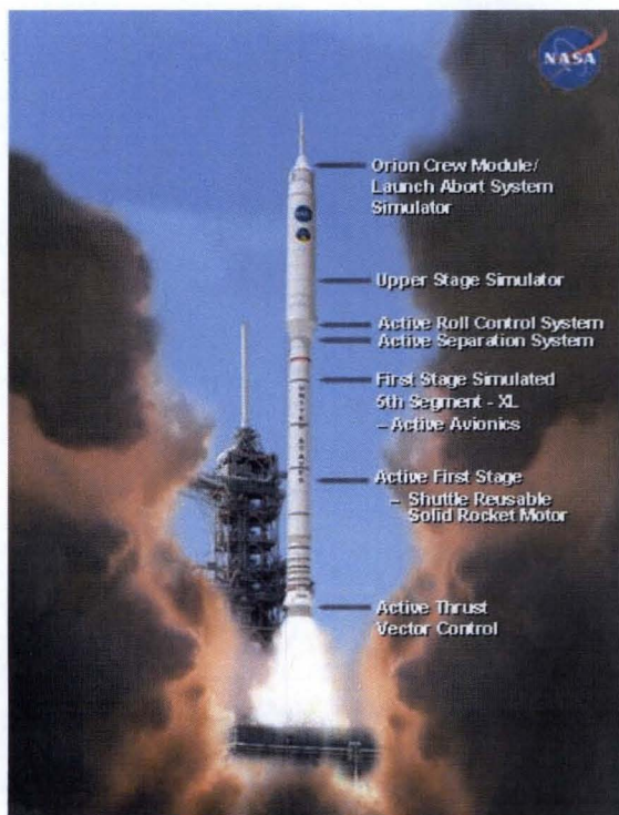
Figure 1. The Ares I-X Flight Test Vehicle incorporates both flight-like and mass simulator hardware.
