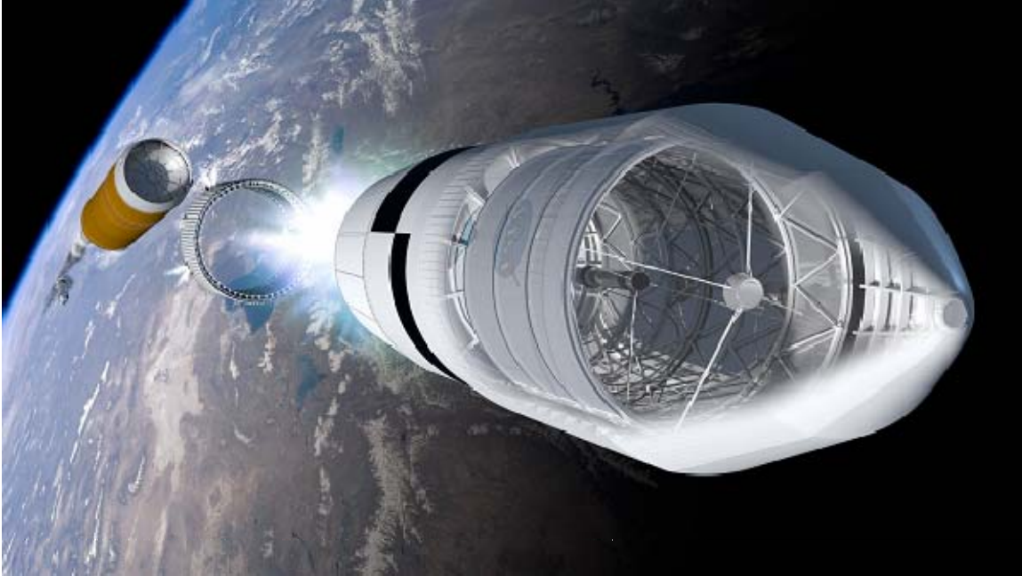
Figure 11. In this artist's conception, Ares V places a monolithic 8-m UV-visual telescope on a path to the Sun
