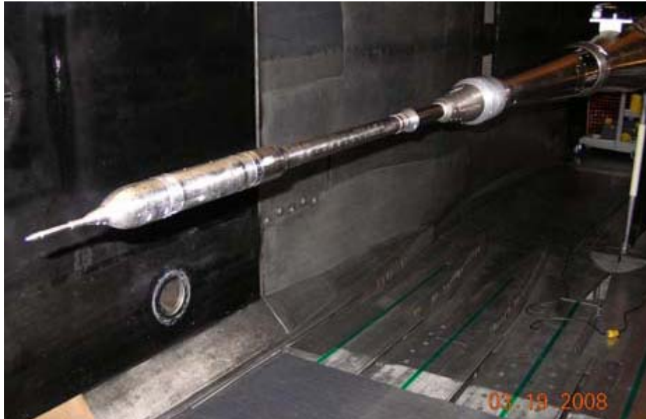
Figure 6. 1% scale pressure model inside the wind tunnel
