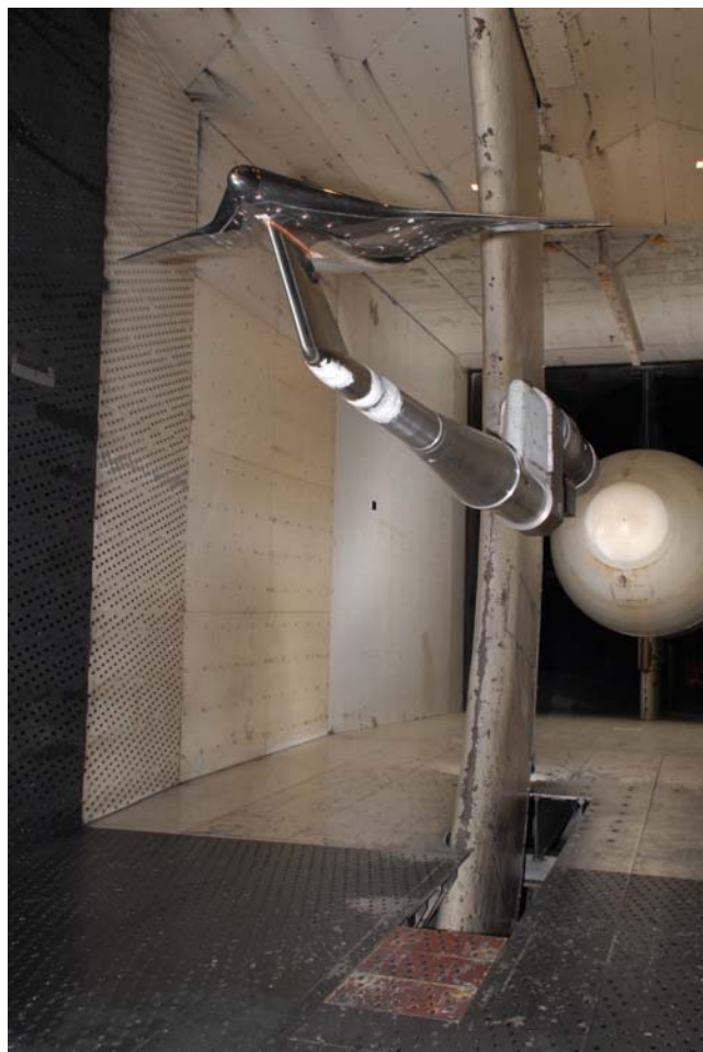
Fig. 10 Installation of 2% BWB model in AEDC 16T (Wing only configuration).
