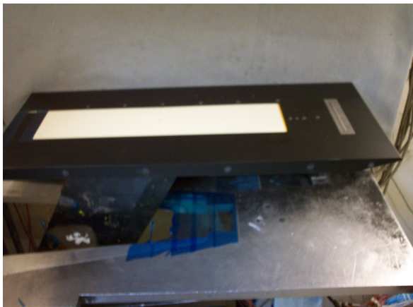
Figure 2. Baseline model with 4-inch by 18-inch ceramic inserts used in Mach 6 for T6888.
