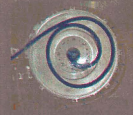
Window inside gimbal; Bundle cable inside.
