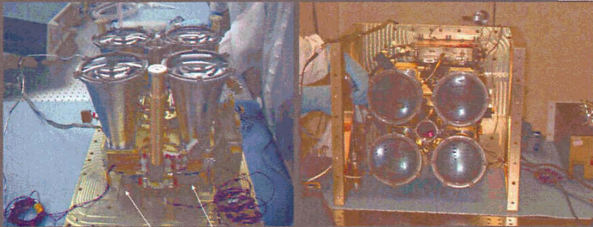
Receiver telescopes focused into optical fiber assemblies that route to different detectors. The MLA is aboard MESSENGER currently sending data from Mercury!
