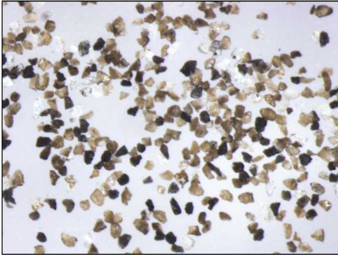
Figure 11.—Photomicrograph of JSC-1AF lunar simulant. Note that most of the particles are transparent.
