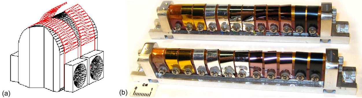
Figure 38. Flexural Stress Experiment: a). Illustration of sample mounting and failure, and b). Pre-flight photo of mandrels.
