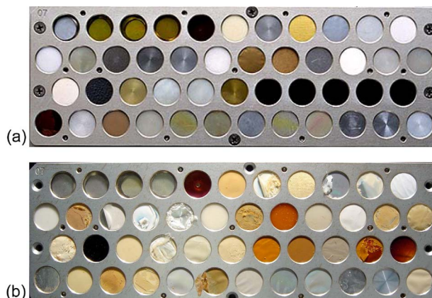
Figure 7. MISSE 2 PEACE Polymers experiment (Sample Tray E5), a). Prior to flight, and b). After space flight.
