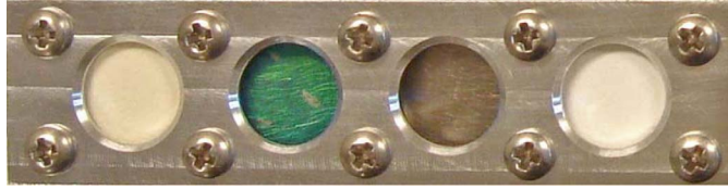
Figure 26. Pre-flight photograph of one set of Cermet Coatings and Thermal Control Paints Experiment samples.
