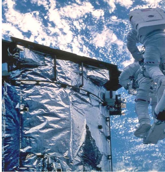
Figure 3. Large cracks in HST MLI after 6.8 years in space.
