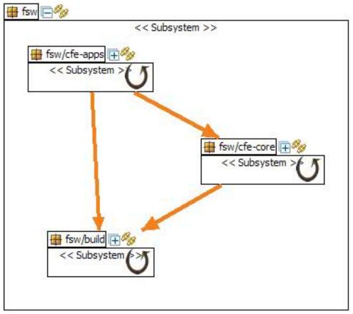
This implemented view is consistent with the design guideline: *Cfe-app* should use *Cfe-core*, but not vice-versa
