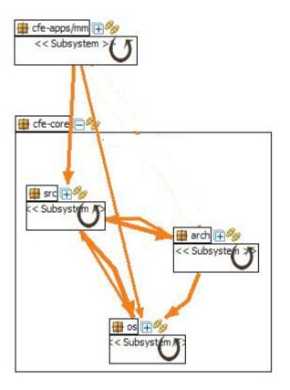
Problem: mm\_load.h directly uses os by directly including "osapi-os-filesys.h"
