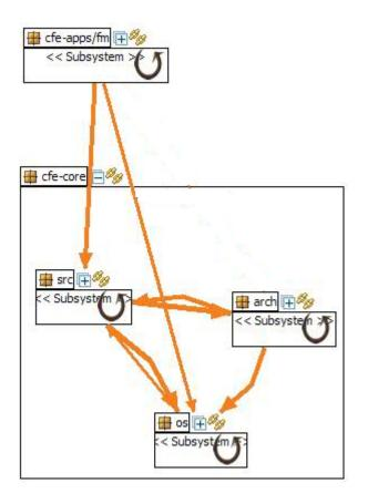
Problem: fm\_cmds.c directly uses os by directly including "osapi-os-filesys.h"
