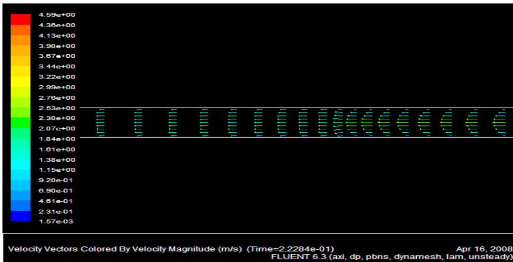
Figure 16 (f) Zoom in on velocity field plot at HXer end. Fluent Grid = 147x56, \Delta t = 6.19E-04 , (480 tpsc); Maximum piston velocity toward the 90° before TDC; Operating Maximum piston velocity toward the 90° before TDC; Operating Conditions: 201.7 RPM, 1.008 MPa).
