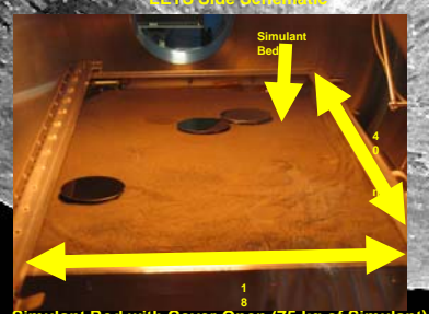
Simulant Bed with Cover Open (75 kg of Simulant)
