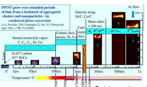
Nanotube nucleation occurs in the 100  $\mu$ s – 1 ms time frame, from carbon clusters and catalyst vapor.
