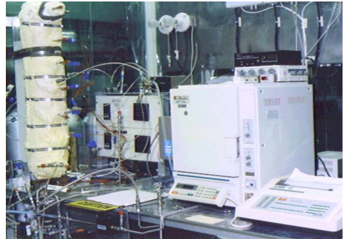
Figure 13A: The test apparatus used for determination of the heat transfer coefficient between the fluid and the sorbent and the fluid and the wall.
