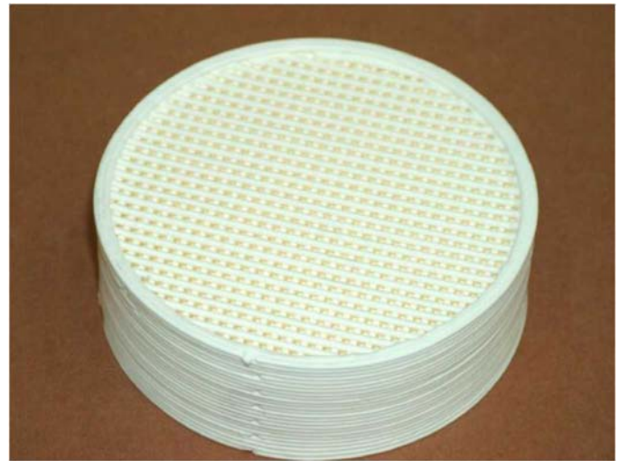
Figure 9: Activated alumina formed by Robocast 6
