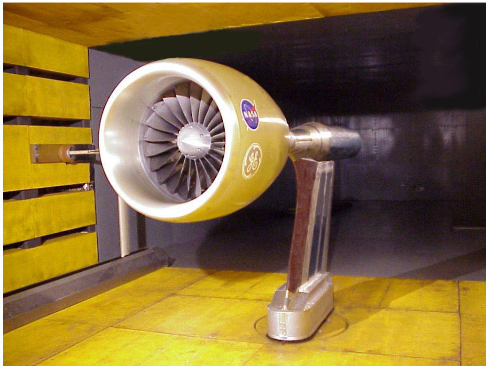
Figure 3.—22-in. scale model of the Source Diagnostic Test (SDT) model fan installed in the 9-ft by 15-ft LSWT.
