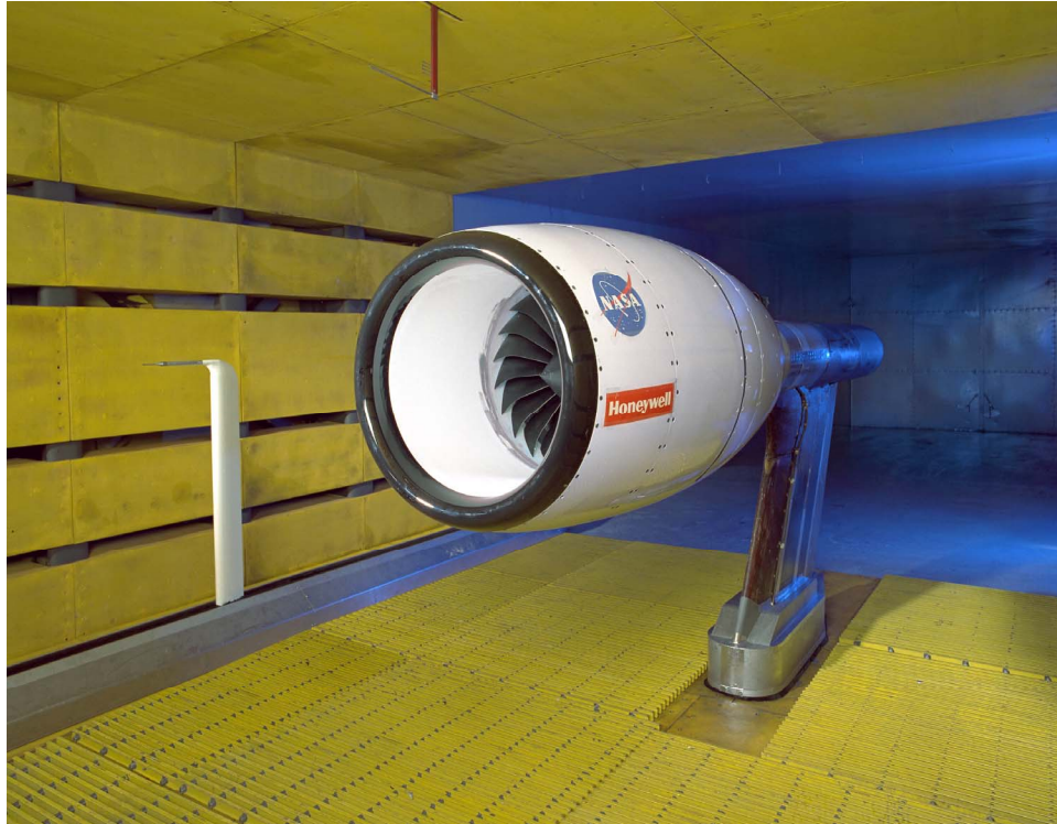
Figure 5.—22-in. scale model of the Quiet High Speed Fan 2 (QHSF2) installed in the 9-ft by 15-ft LSWT.
