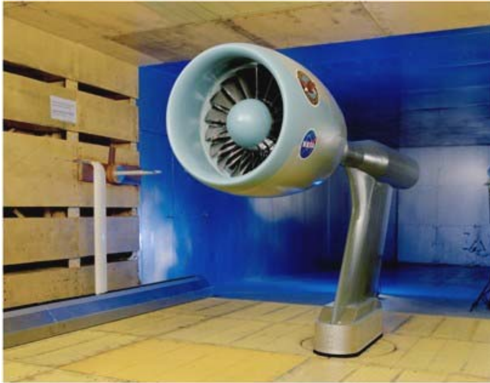
Figure 1.—22-in. scale model of the Advanced Ducted Propulsor (ADP) Fan 1 installed in the 9-ft by 15-ft LSWT.
