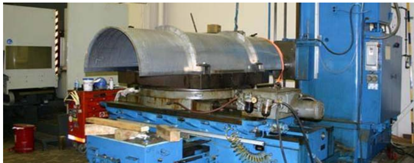
Figure 15. The LAS tube section is in the midst of fabrication
