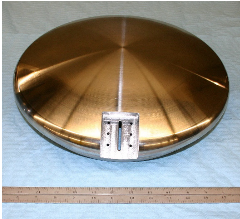
Figure 14: Final Machining of 67-CH Heat Shield Section
