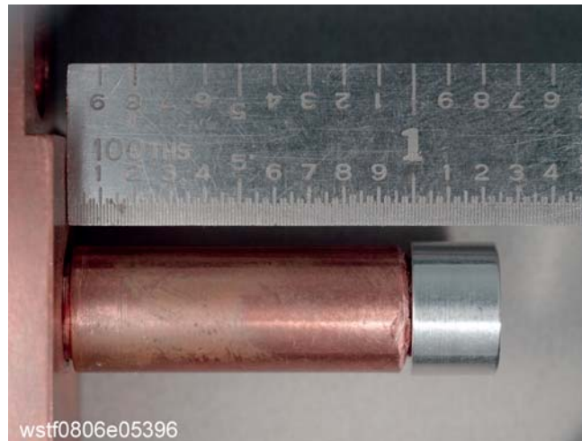
FIG. 6—Standard supersonic target configuration.
