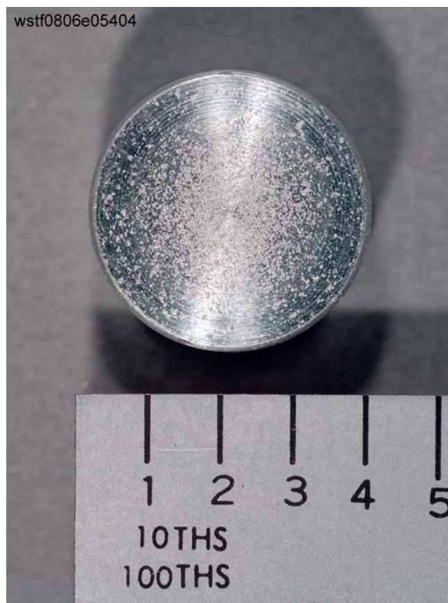
FIG. 20—Typical supersonic target test results of a no burn with aluminum (Test Series 6).
