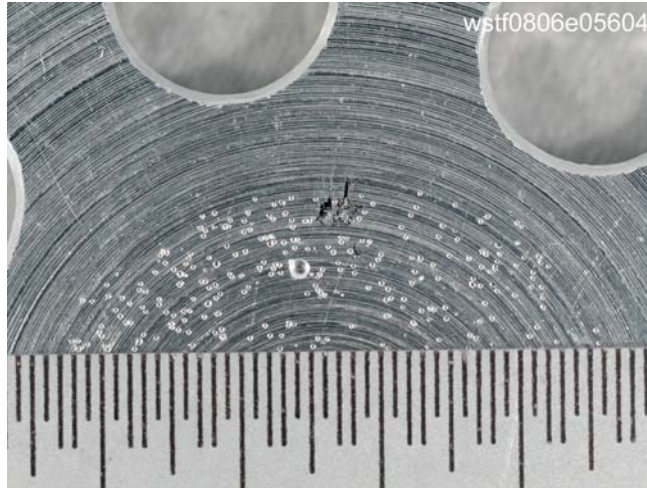
FIG. 10—Typical subsonic flat target test results of a particle burn with titanium (Test Series 1).
