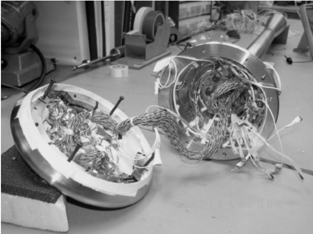
Figure 6. Disassembled CEV model heat shield and aftbody
