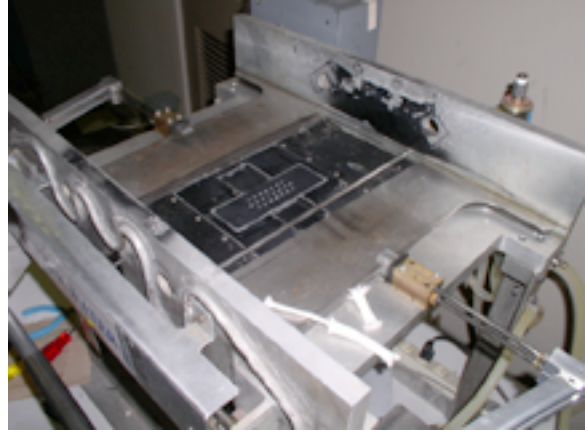
Installed Sample Plate (shutter and lamp removed)
