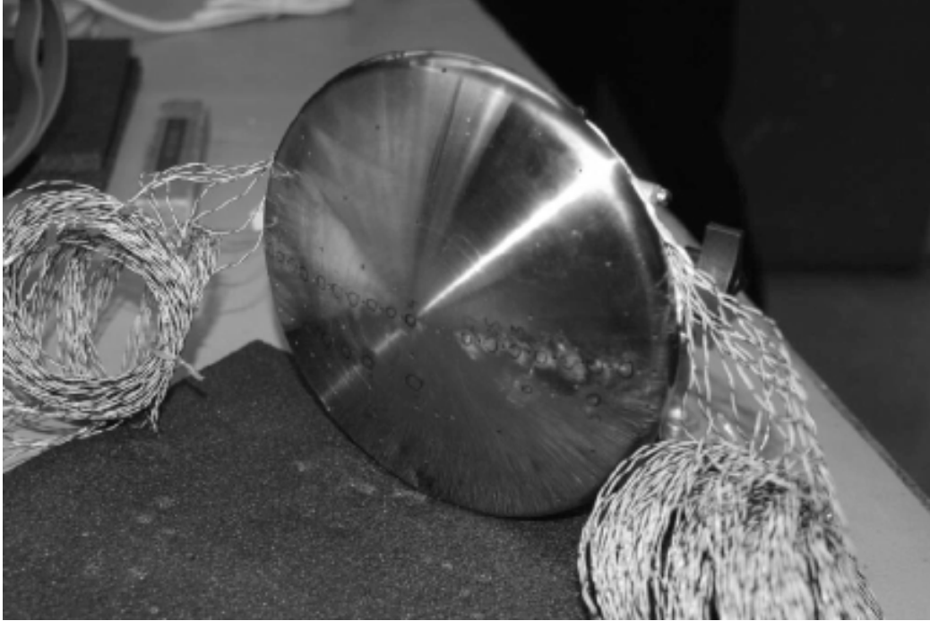
Figure 5. CEV model heat shield during thermocouple installation process
