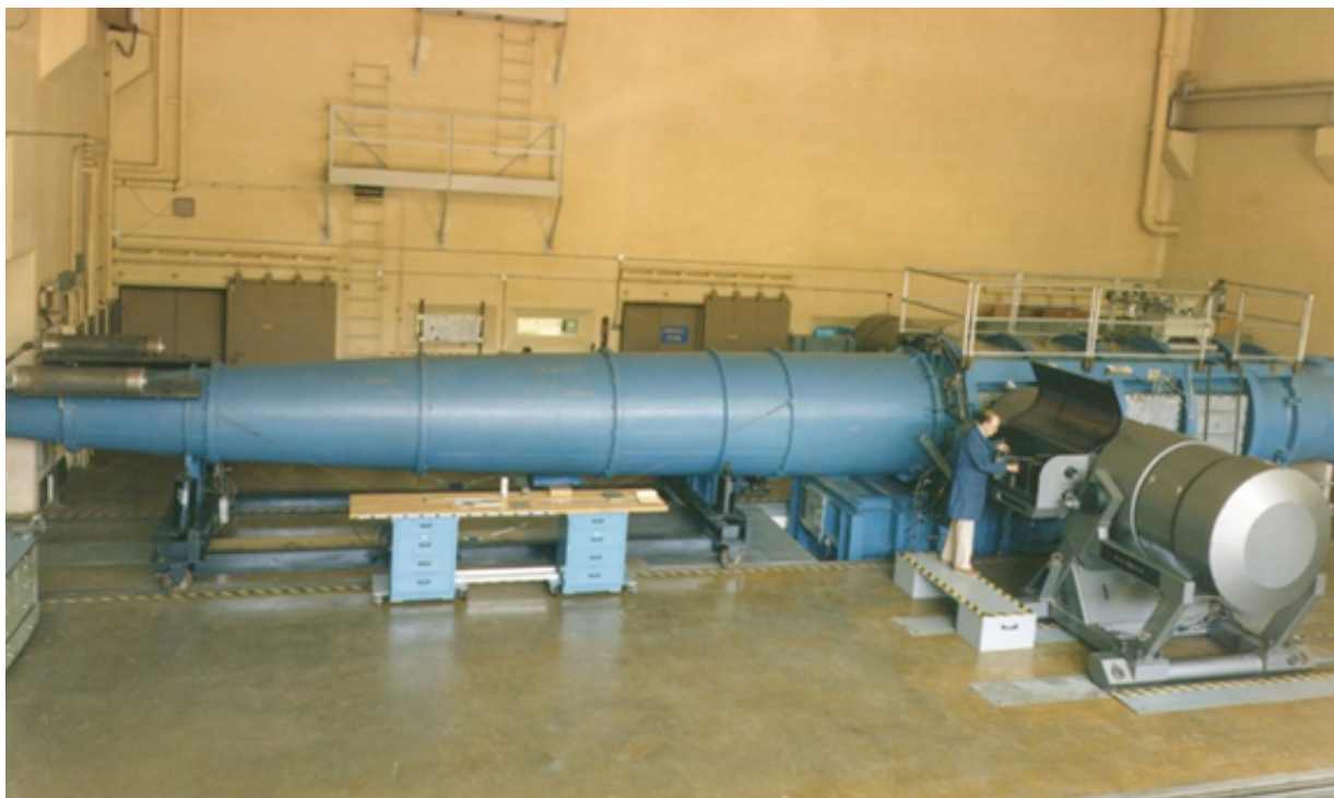
Figure 8. AEDC Hypervelocity Tunnel 9 (Mach 10 nozzle)
