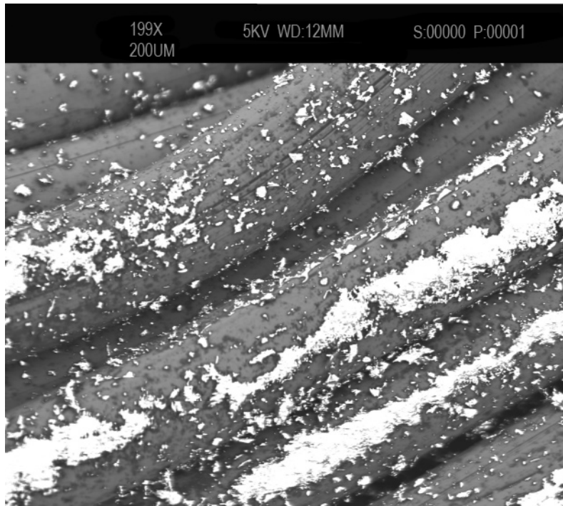
Figure 5. High-magnification image of wire showing the presence of contamination that is low molecular weight and insulating as indicated by the large amount of charging.
