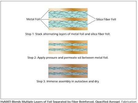
HyMATI Blends Multiple Layers of Foil Separated by Fiber Reinforced, Opacified Aerogel. Fabrication consists of: (a) stacking alternating layers of reflective metal foil and high purity quartz fiber, (b) applying slight pressure to the stack to control the spacing between metal foil layers, and (c) permeating the liquid aerogel precursor into the stack, followed by solidification and supercritical drying.
