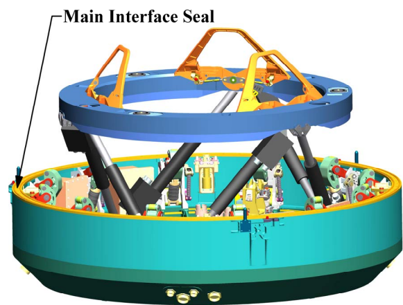
Figure 2. Schematic of an active LIDS and main interface seal.
