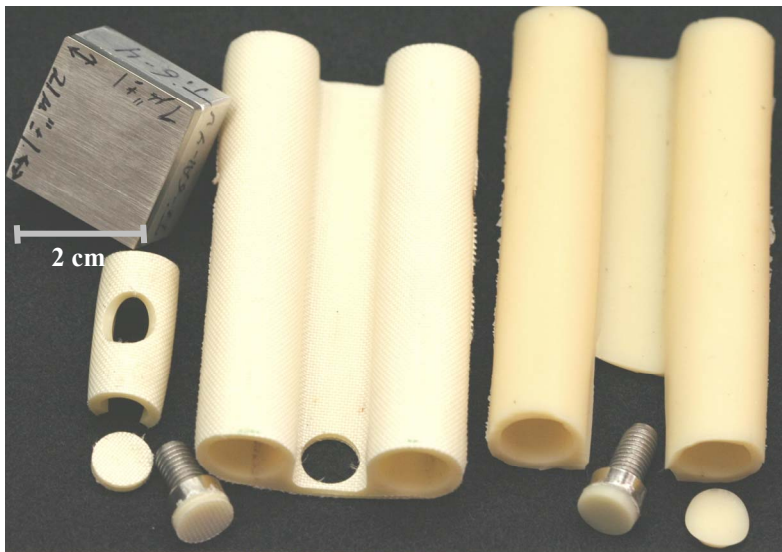
Figure 6. Image of hollow heat shield seals being considered for CEV applications. The seal on the left was covered with a Nomex heat resistant cloth during manufacturing. Buttons cut from the seal were adhesion tested.
