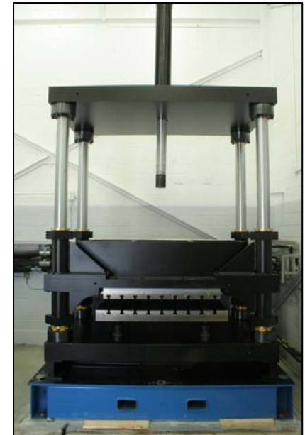
Full-scale actuated LIDS seal test rig
