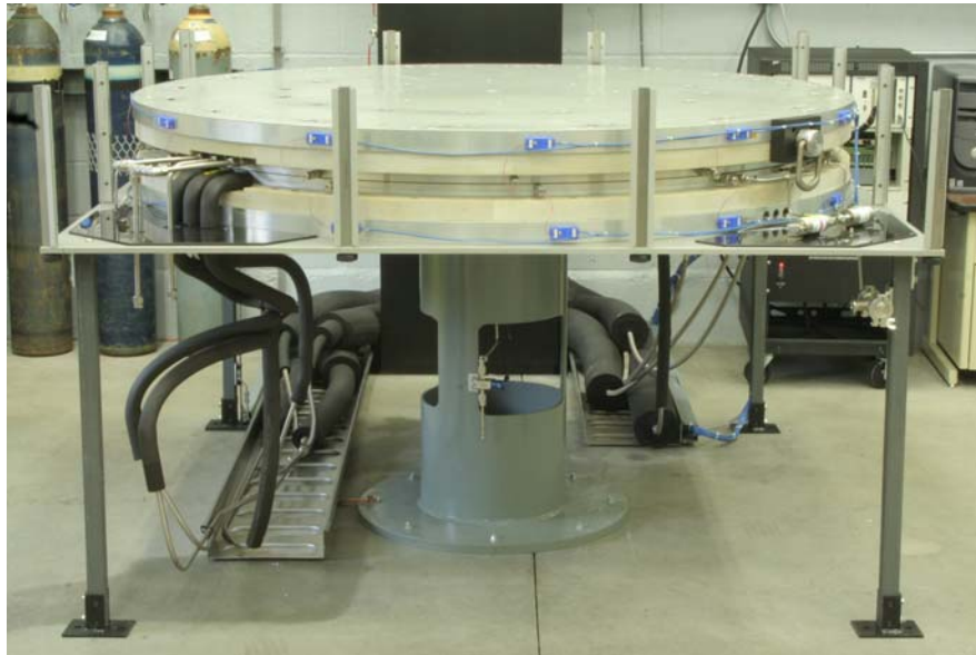
Full-scale non-actuated LIDS seal test rig
