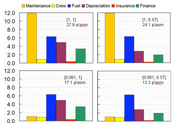
Figure 12. Cost elements compared for LCTR with and without cost technology factors lift rotorcraft (1200 nm, 120 passengers); in legend [x,y], x is maintenance factor and y is price factor.
