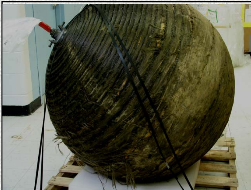
Columbia OV-102 COPV (40 inch) Model S/N 029 Damaged Outer Shell
