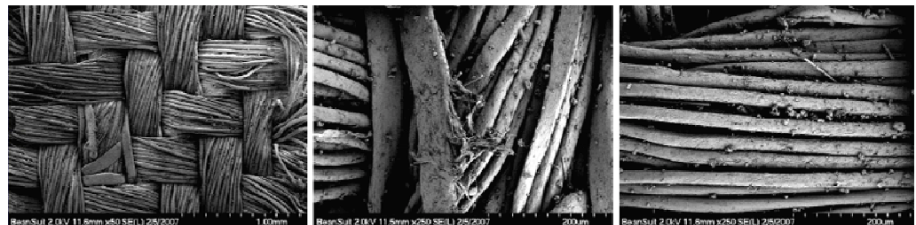
Electron micrographs showing damage to the outer layer of Alan Bean's Apollo 12 suit.
