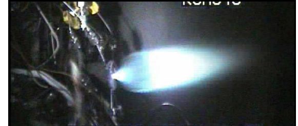
RCE Class Igniter Vacuum Testing – GRC RCL21
