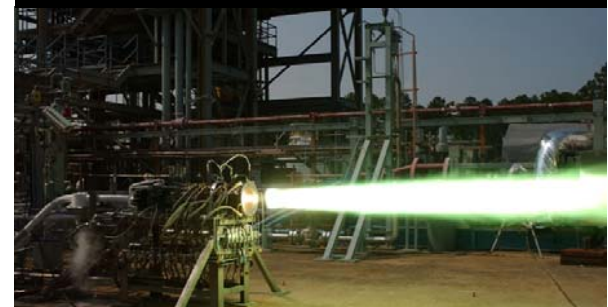
6" Injector Hot-fire Test (Ablative Chamber), MSFC TS115
