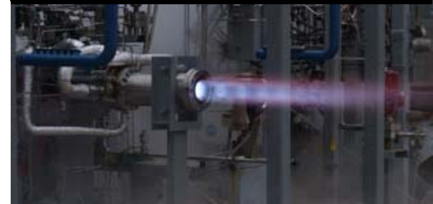
6" Injector Hot-fire Test (Ablative Chamber), MSFC TS115
