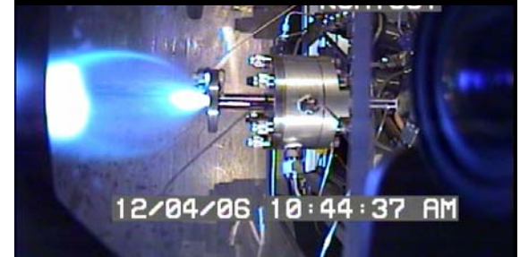
Main Engine Class Igniter Vacuum Testing – GRC RCL 21
