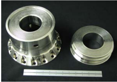
Figure 5 Heater head and cooler assemblies
