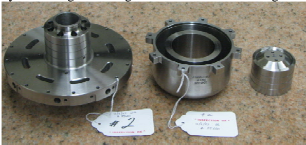
Figure 6. Displacer drive components: post and flange, gas spring cylinder, gas spring piston (l to r)
