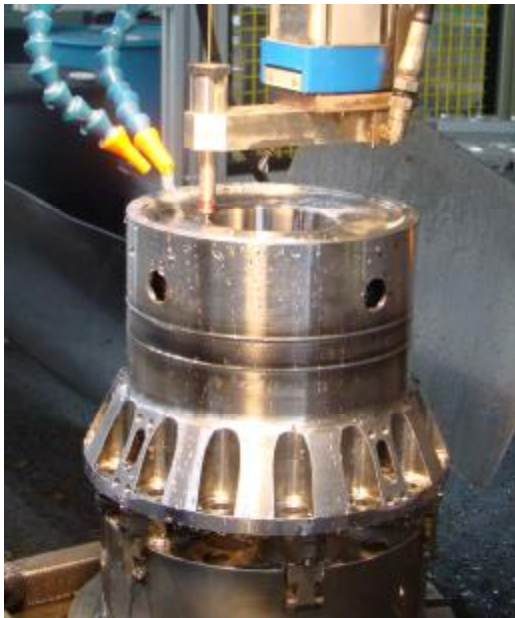
Figure 3. Heater head machining process. Holes for the heater head tubes are drilled using an electrodischarge machining (EDM) process.
