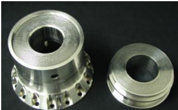
Figure 2. Heater head and cooler assemblies. Assemblies are shown prior to electron-beam welding of tubes.
