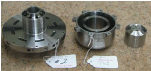
Figure 4. Displacer drive components. Shown left to right: post and flange, gas spring cylinder, gas spring piston.
