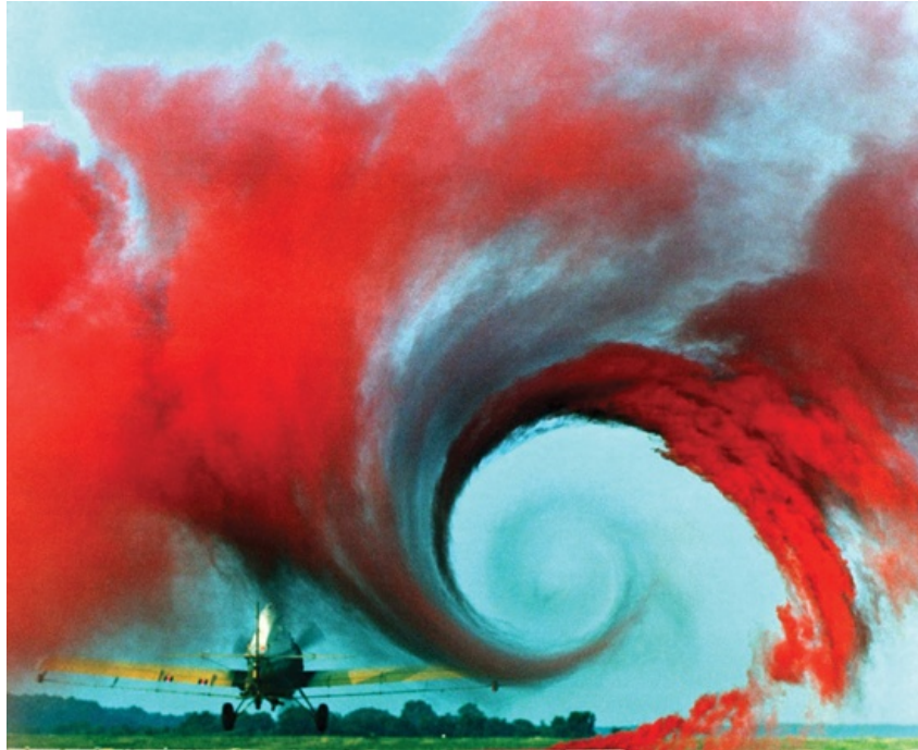
Figure 36. Example of red-colored smoke entrained in wake of aircraft.
