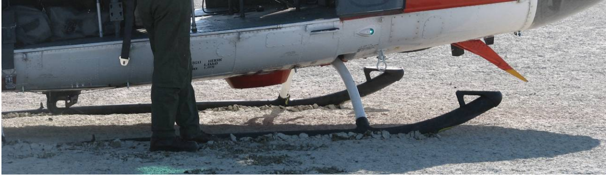
Figure 6-7: Huey H1 helicopter legs sinking into Carson Sink. The H1 weighs approximately 10,000 lbs.
