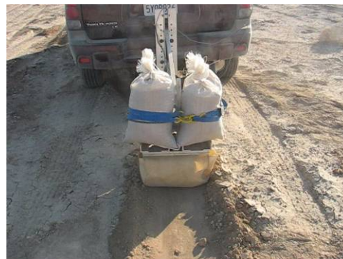
Figure 5-3: ~280 lb loaded airbag drag causes some plowing
