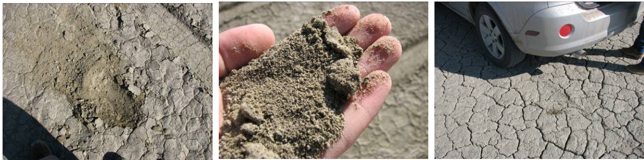
Figure 6-4: (left) Surface “flakes” from Carson Sink’s cementation. (center) Close up of Carson Sink soil, can be squeezed to form cohesive chunk. (right) After driving over, it is observed that drier portions of Carson Sink behave as stiff as Cuddeback Soil A.
