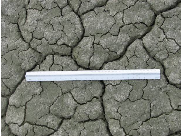
Figure 6-5: (left) Drier Carson Sink areas were hard and appear cracked. (right) Wetter areas appeared almost completely smooth and significantly displaced under load.
