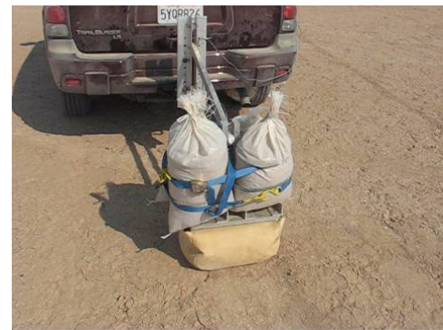
Figure 4-8: Airbag drag on Soil A. Note the lack of deformation behind the bag.
