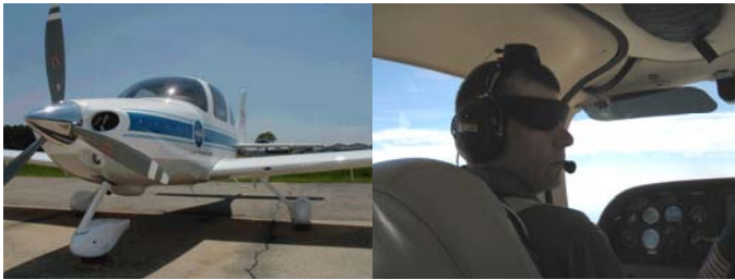
Figure 1. Left panel: NASA's Cirrus SR-22X aircraft, used as the experimental testbed. Right panel: Subject pilot wearing vision obscuring goggles.
