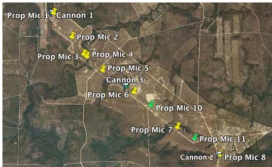
Figure 6. Propagation test configuration.
