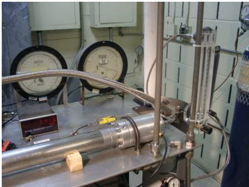
Figure 2.—Pressure gauges and flowmeter.
