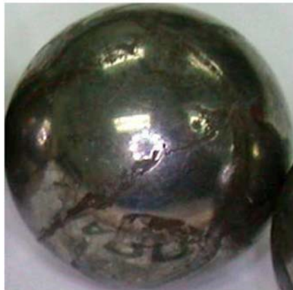
Figure 11.—Oil cooler fan bearing damage.
