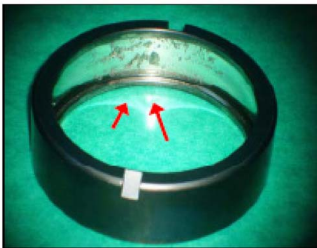
Figure 16.—Damage to the outer race.
