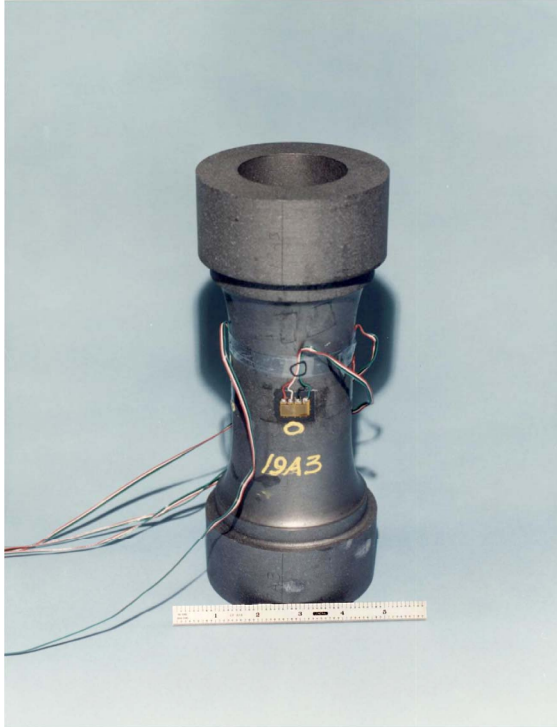
Figure 6.—Oak Ridge National Laboratory multi-axial specimen with strain gauges.
