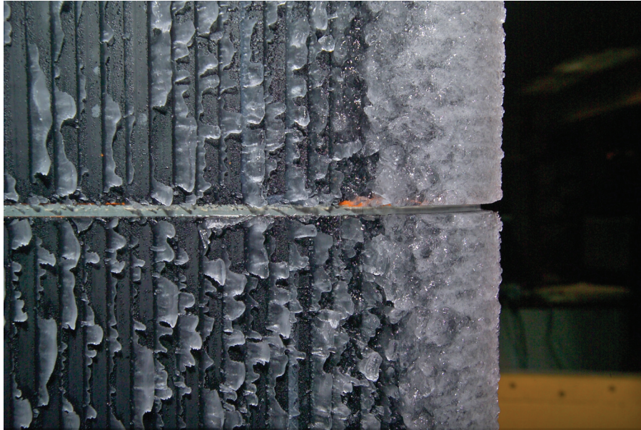
Figure 4.—Photograph of lower surface ice for case EG1328.
