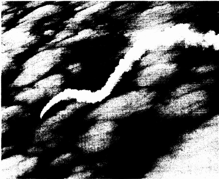
NASA Dryden Flight Research Center Photo Collection http://www.dfrc.nasa.gov/gallery/photo/index.html NASA Photo: EC01-0182-11 Date: June 2, 2001 Photo by: Jim Ross The X-43A/Pegasus combination dropped into the Pacific Ocean after losing control early in the first free-flight attempt.
