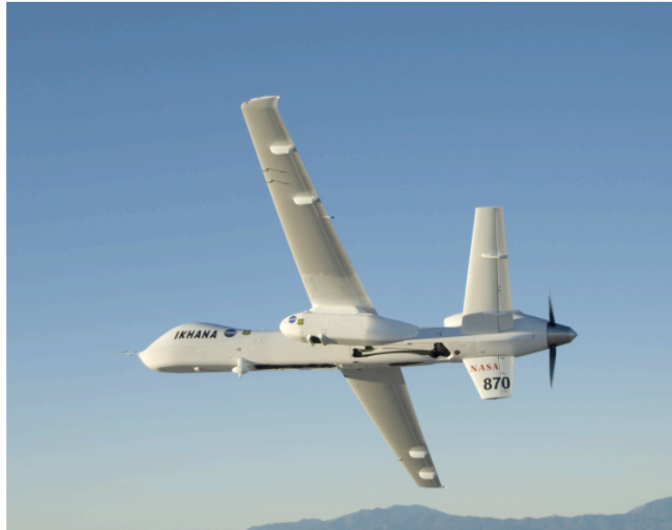
Fig. 6. The Ikhana aircraft carrying the fire pod.
