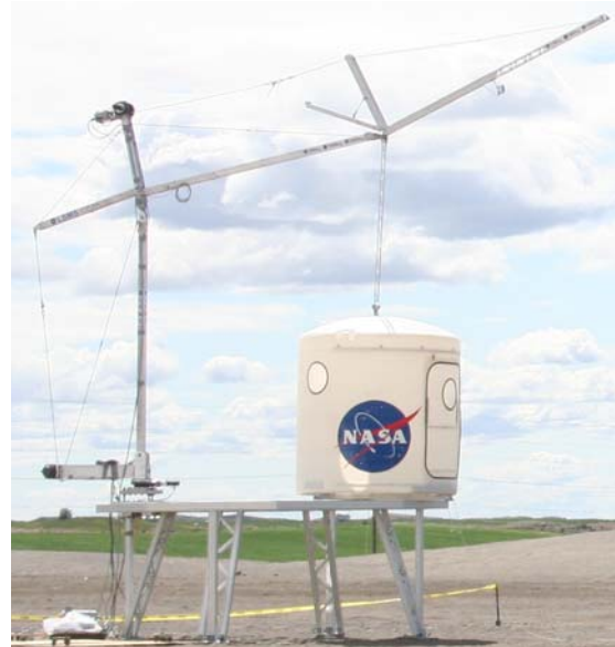
Figure 16. LSMS on Elevated Platform Preparing to Offload Large Airlock Mockup.
