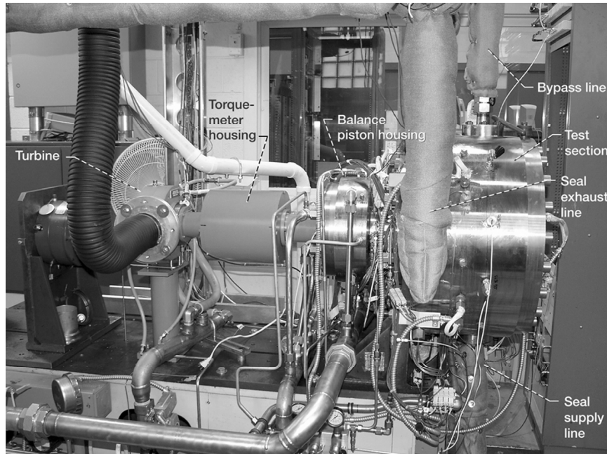
Figure 1.—NASA's Turbine Seal Test Facility.
