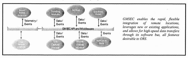
with advance time for safe evacuation. Additional application components can be brought on-line as quickly as required to interpret the results from the field. Better yet, other remote locations can be added to the message bus middleware as needed to enhance the data acquisition. This scenario is illustrated in the figure below.
