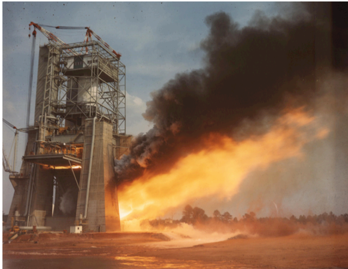
Fig. 8. Marshall's Static Test Stand (TS-4670) accommodates large rocket engine testing, such as the Saturn V cluster of five F-1 engines.
