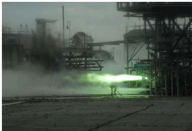
Fig 6. J-2X subscale main injector hot-fire testing at Marshall.
