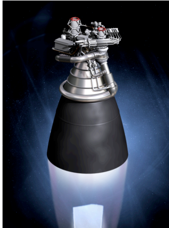
Fig. 10. Concept of the J-2X engine.
