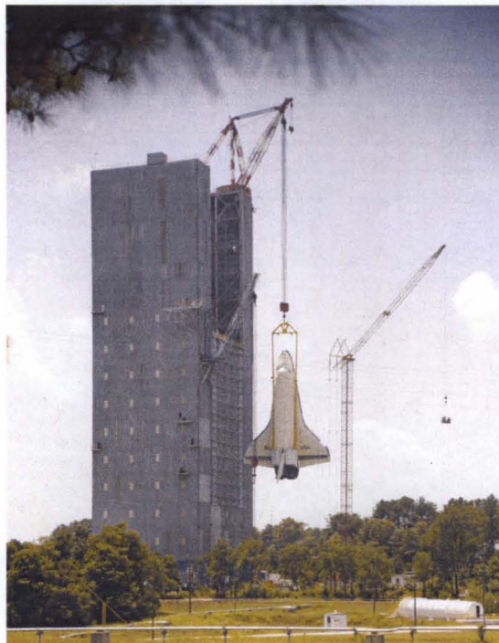
Fig. 2. Marshall's Dynamic Test Stand was used to gather ground vibration test data prior to flying the new space transportation system.
