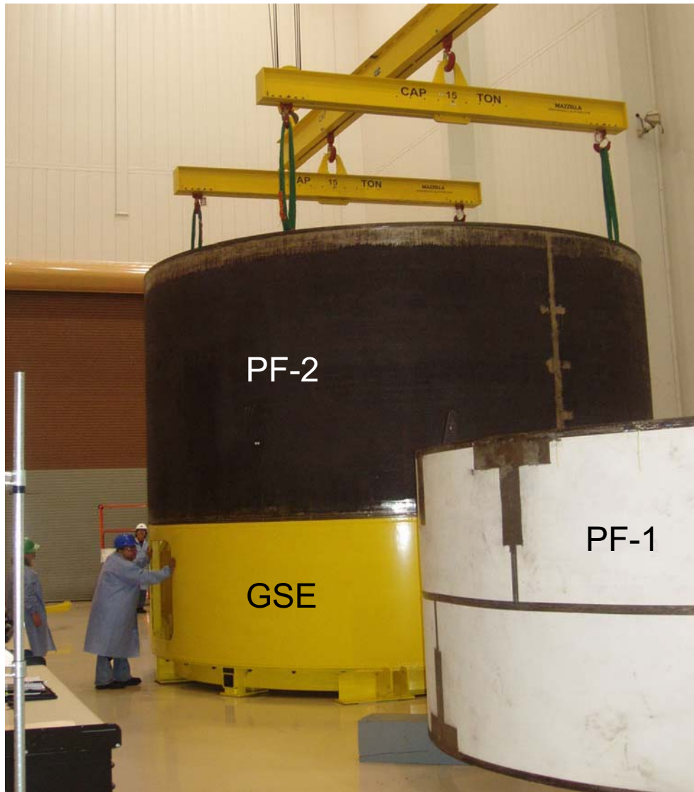
Figure 81. Segment mating test using pathfinder USS shell segments (NASA Glenn photo).
