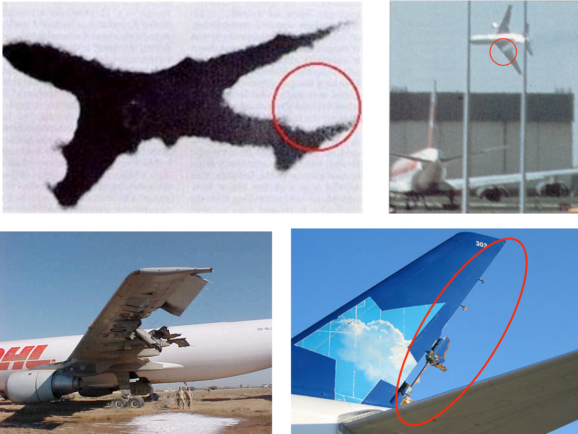
Figure 1. Examples of transport aircraft damage (clockwise from top left): B747 Vertical Tail Loss 2 ; DC-10 Engine Loss/Asymmetric Slat 1 ; A310 Rudder Loss 6 ; A300 Wing Damage 5
