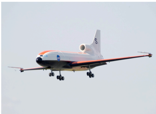
Figure 2. S-2 subscale jet transport aircraft.
